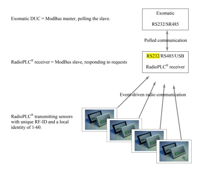
The ModBus communication might be possible to run simultaneously with the RadioPLC<sup>®</sup> terminal mode, thus simplifying test, setup and field service.
